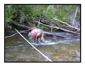
Figure 8. Measuring depth and substrates along a channel transect.
