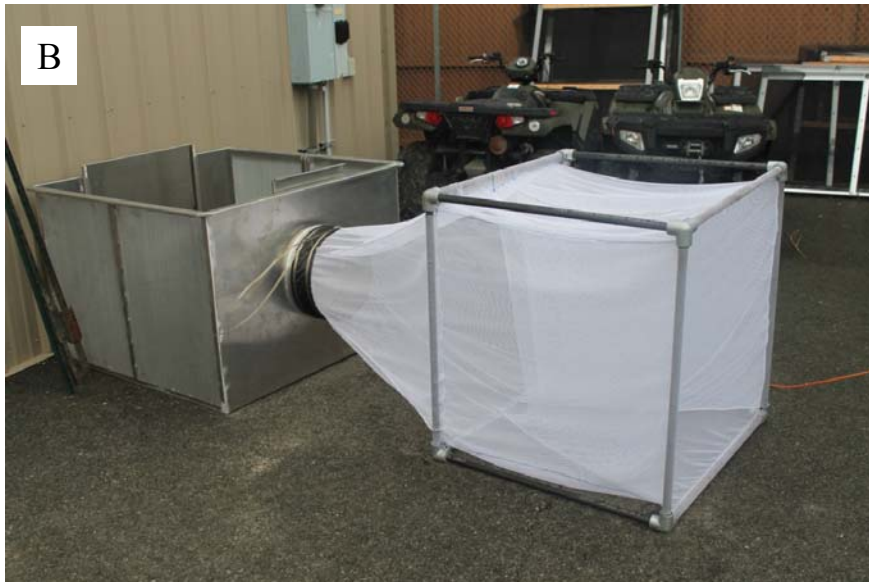
Figure 3. Modified double frame fyke net showing; (A) internal winkers and tapered cone affixed to trap live-box and; (B) live-box with perforated plate sides and removable back panel.
