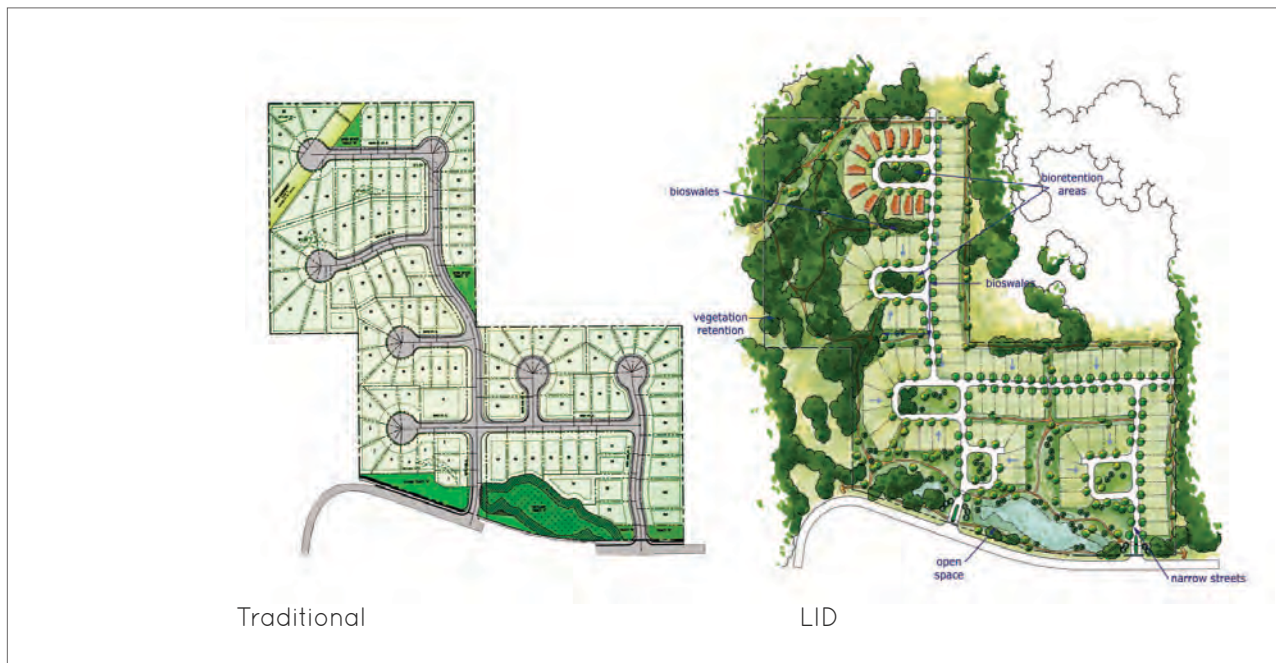
Figure 9. (below) Comparison of a traditional development layout with one that incorporates low-impact development techniques.
