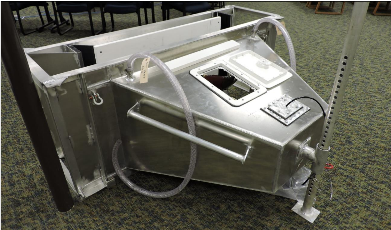
Figure 6: Video weir camera box and passage chute.
