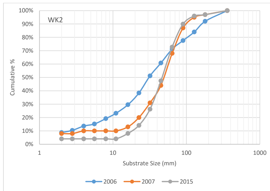
Figure 4. Substrate size distribution at the treatment WK2 site comparing previous and current measures.
