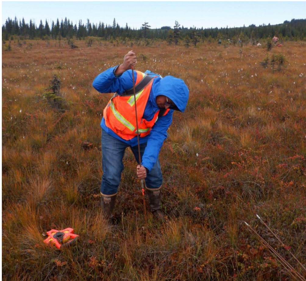
Figure 17. A researcher measuring peat depth with a tile probe. Peat depth is a useful proxy for the amount of organic material in the surrounding peatland zone.
