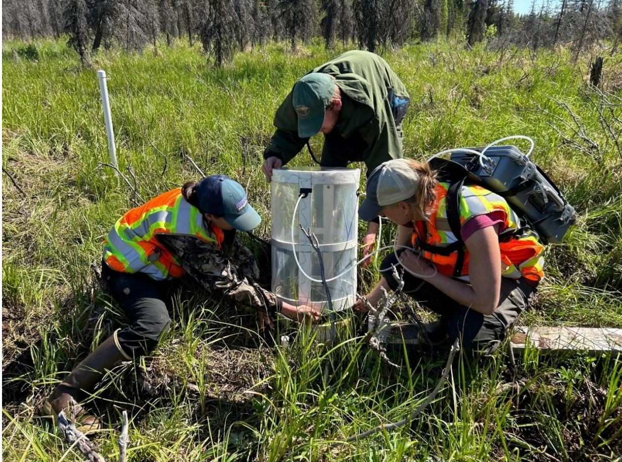
Figure 24. Researchers set up a gas flux chamber in a wetland near Happy Valley, Alaska. The LI-7810 analyzer is connected to the chamber via tubing; the researcher on the right carries the analyzer as a backpack. Containing the gas flux analyzer in a plastic tote during field use offers it more protection and frees up researchers during data collection.
