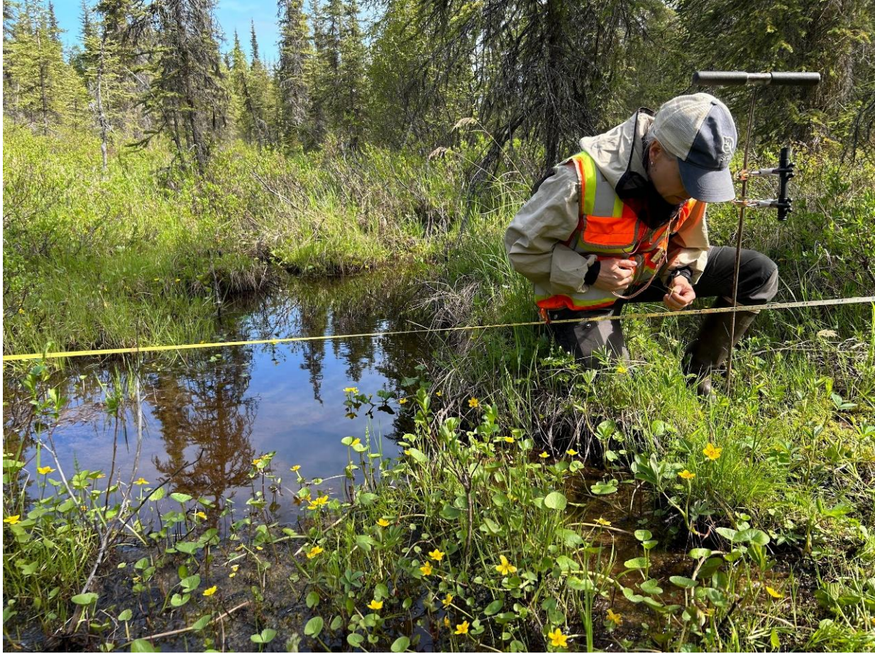
Figure 5. A researcher using a transect tape and vertically-mounted laser pointer to survey vegetation using line point intercept methods. These methods reduce bias as compared to a visual survey and enable the calculation of both foliar cover and top cover.
