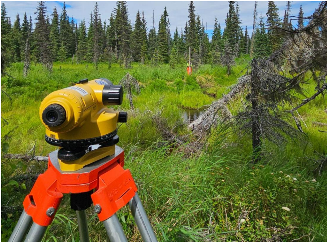
Figure 13. Elevation can be surveyed using an auto level (foreground) and a stadia rod (background). Once the auto level itself is level, direct the eyepiece at a “benchmark” with a known, possibly arbitrary, elevation that is marked in the field for future reference (for example, a triangle cut into the bark of a tree). Determine the height of the level relative to the benchmark by viewing the stadia rod (held vertically with the base at the benchmark) through the eyepiece. Determine subsequent well elevation(s) by turning the eyepiece horizontally and viewing the height of the stadia rod above the well(s). Well elevations can then be calculated relative to the benchmark elevation. If needed, the height or location of the auto level can be adjusted using a “turning point,” which involves resurveying a known point (e.g., the last monitoring well surveyed) with the new auto level configuration, then continuing with subsequent measurements. Photo credit: USF-ERG.
