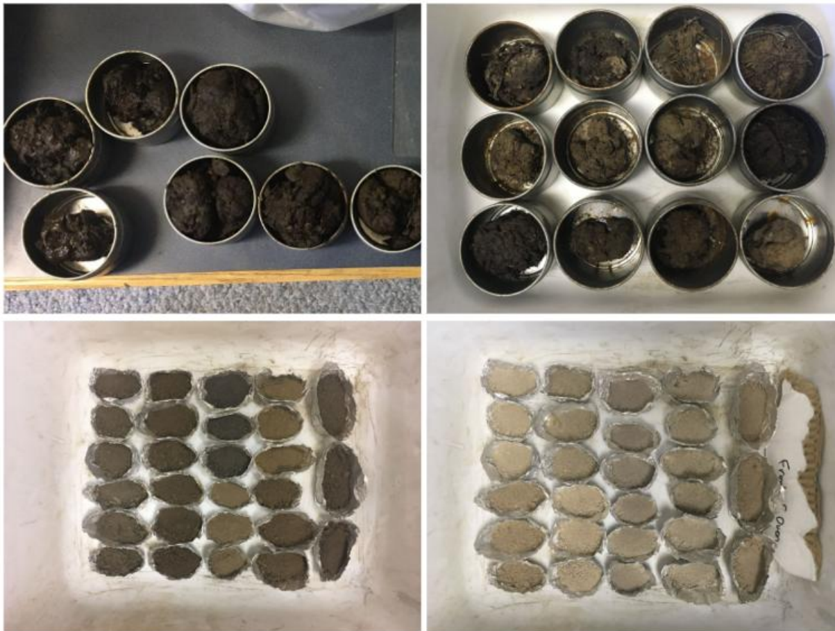
Figure 23. Wet peat in aluminum cups (top left), dried peat in aluminum cups (top right), dried and ground peat in foil boats prior to loss on ignition (bottom left), and ash remaining after loss on ignition (bottom right).
