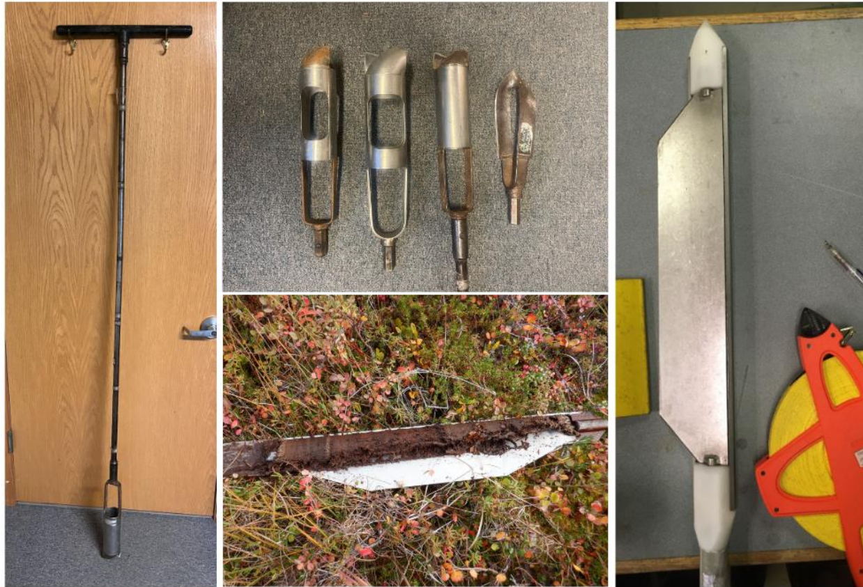
Figure 18: Bucket auger and Russian peat auger. Note that different auger heads (top center) can be attached to the bucket auger (left); the Dutch auger style (top center right) often works best for peat. Each of these heads is made to be twisted down into the soil. In contrast, the Russian auger has a pointed head (right) that is driven directly down before turning the auger 180 degrees around the fin; opening up the fin reveals the half-cylinder sample (bottom center).
