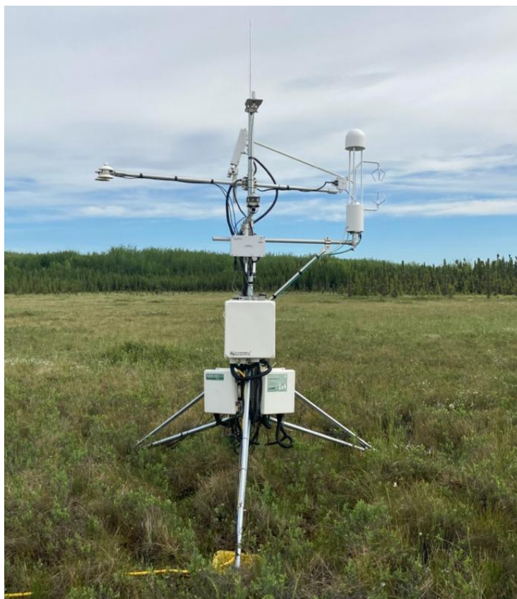
Figure 25. Eddy covariance tower at Lily Lake Fen in the northern Kenai Lowlands. The tower measures carbon dioxide and methane flux, and how these fluxes vary over time.
