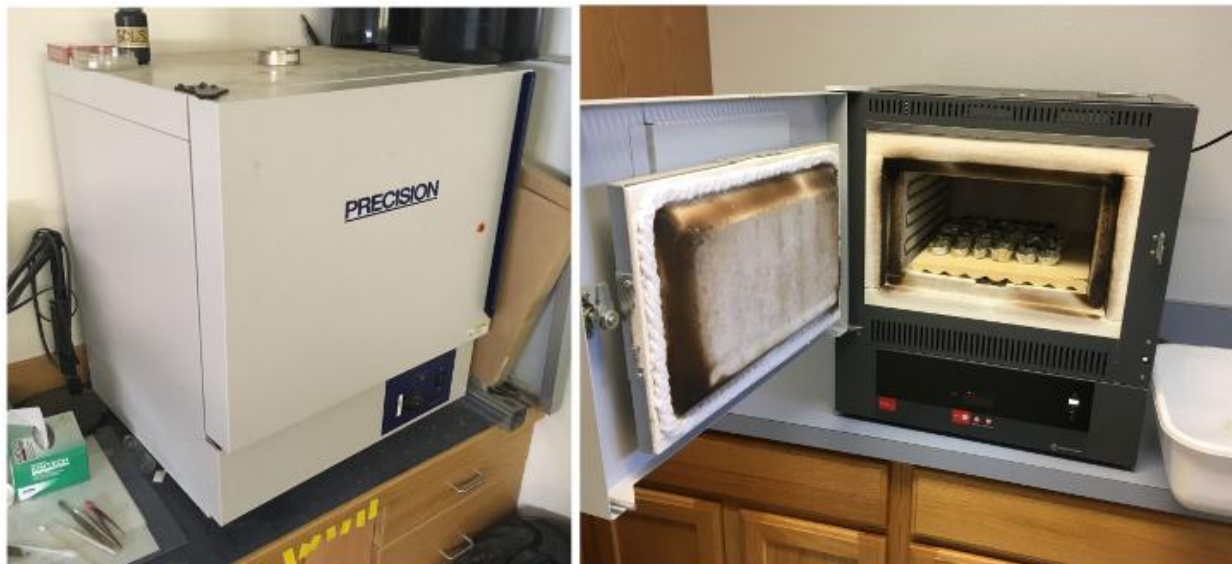
Figure 22. Laboratory oven (left) and muffle furnace with soil samples (right). The oven is typically used for drying samples, while the muffle furnace (which can get much hotter) is used for combustion. This procedure uses both instruments.
