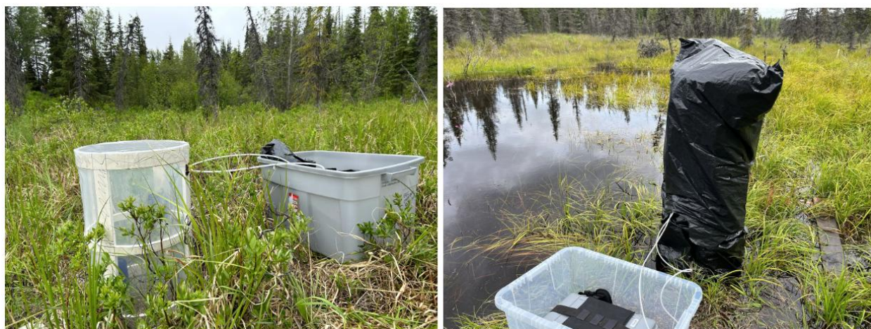
Figure 17. Gas flux light reading (left) and dark reading (right) in a freshwater wetland near Happy Valley, AK. The dark reading makes use of an extension chamber due to flooded conditions; note that four plastic bags are used (two for chamber, two for extension) to fully block the light.
