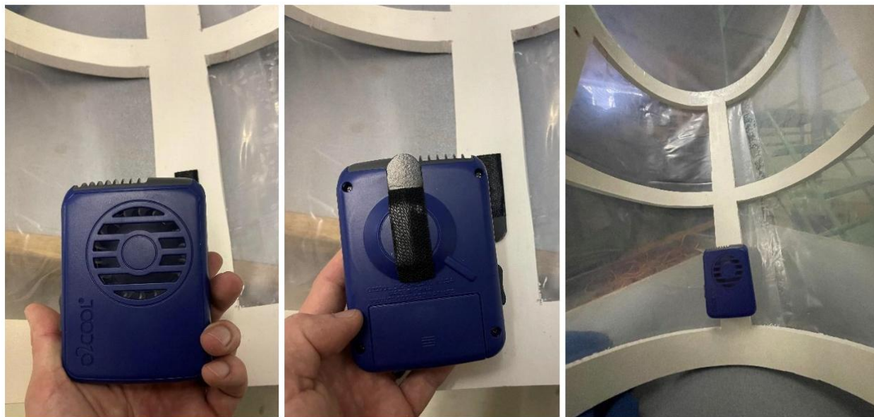
Figure 7. Battery powered fan: front, back, and attached with Velcro on the inside of the chamber.
