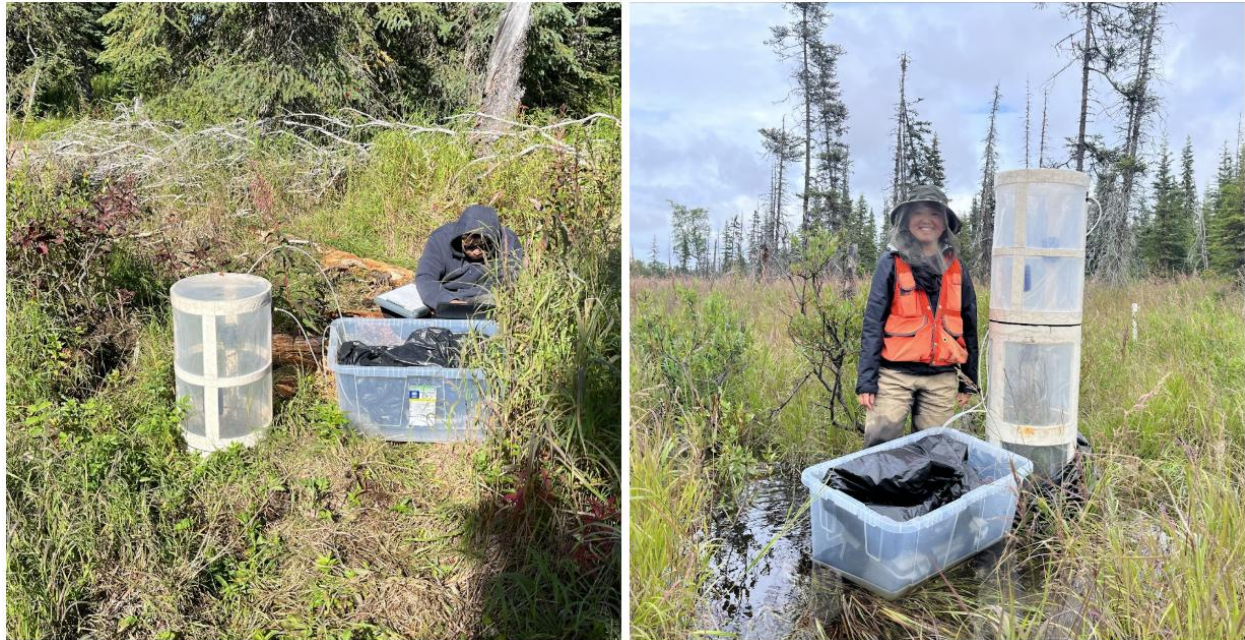
Figure 1. Using the LI-7810 unit with chamber and collar in a freshwater wetland near Happy Valley, Alaska in dry conditions (left) and in standing water (right). Note the plastic tote to protect the unit. In the left photo, a researcher is using a computer to monitor real time data. In the right photo, an extension chamber has been added to accommodate standing water and taller vegetation.
