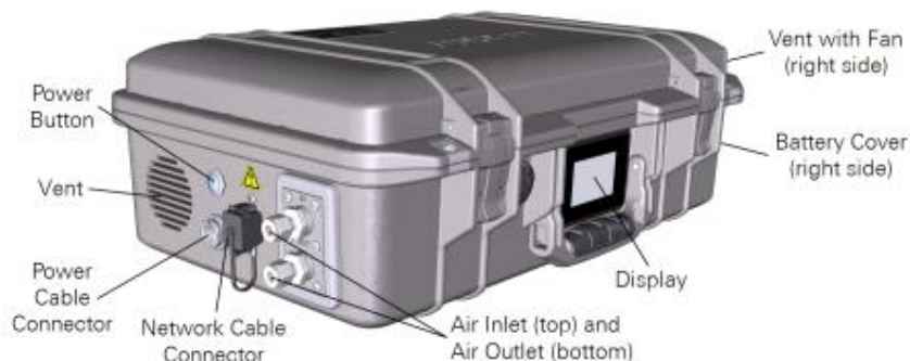
Figure 9. Schematic of the LI-7810 Trace Gas Analyzer (credit: LI-COR Environmental)
