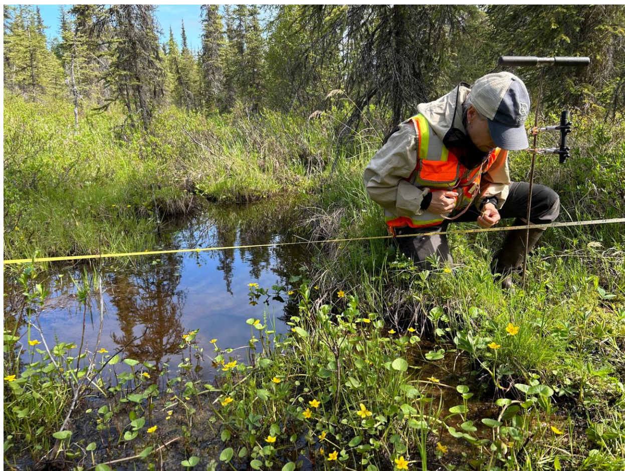
Figure 14. Example of line point intercept methodology using a vertically-mounted laser pointer.
