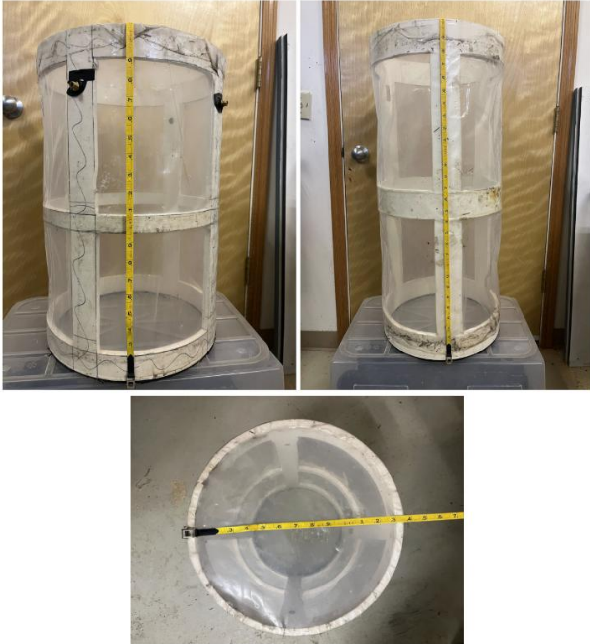
Figure 4. Chamber (top left, bottom) and extension chamber (top right) with greenhouse plastic and weather stripping. Scale shown in tenths of feet.
