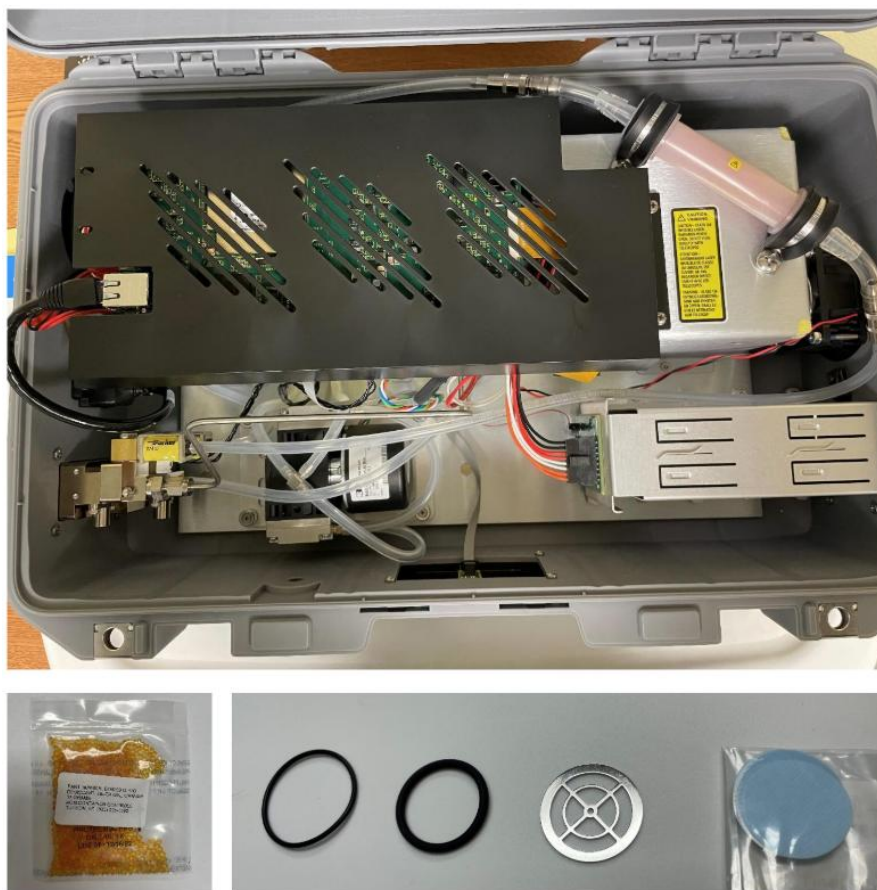
Figure 12. Interior of the LI-7810 unit; desiccant tube filled with orange silica beads is shown in the upper right. Replacement desiccant and air filters and gaskets shown below.
