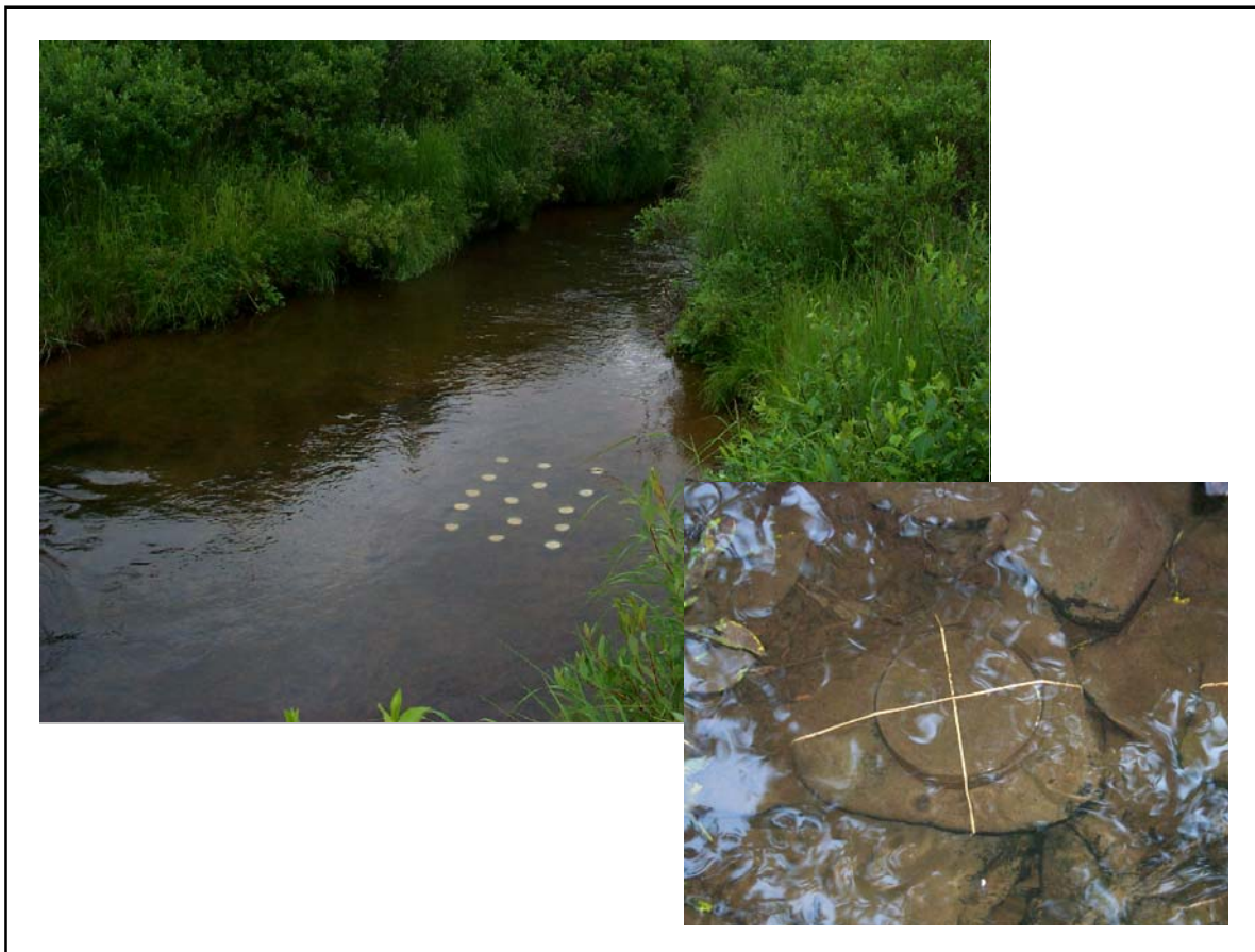
Figure 8. Sediment collector array and (inset) individual sediment collector.
