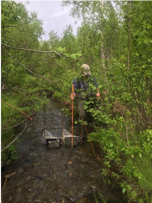
Figure 4. Measuring depth and stream velocity at the mouth of a driftnet deployed in South Fork Chester Creek, June 2017.
