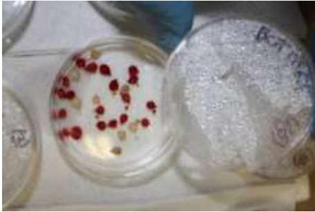
Figure 7. Example of tetrazolium seed viability test results. This test differentiates live, respiring seeds (red) from dead, non-respiring seeds (white) based on color.
